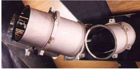
Fig. 3 Astronomical replicated Wolter mirrors for the KORONAS satellite (replicated from one and the same mandrel). Wolter 1, aperture 80 mm, electroformed nickel (single layer). The mount structures were created during the galvanoplastic process in order to improve the mechanical stability and overall stiffness (unique solution). This was the last INTERCOSMOS program X-ray telescope with our participation.
