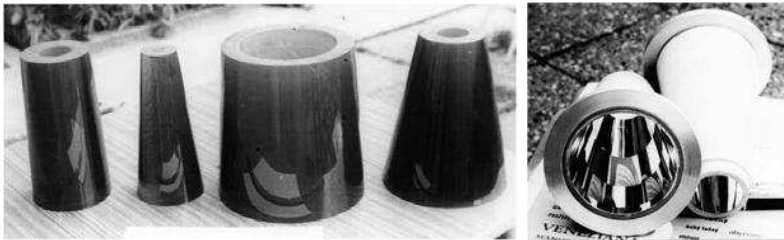
Fig. 2 The four mandrels used for the manufacture of the X-ray mirror nested array for the RT-4M soft X-ray telescope (Glass ceramics Sital). Flown onboard the space station Salyut 7. (left). Two identical mirrors (large hyperbolas) of the RT-4M mirror array (Ni surfaces). (right).
