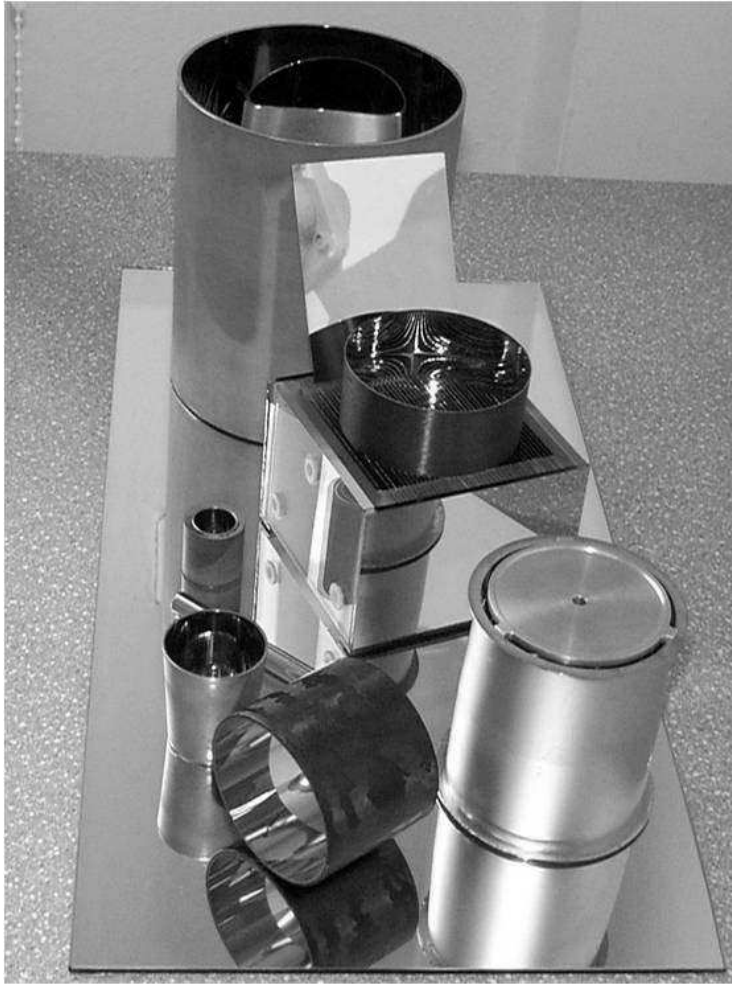
Fig. 1 Various replicated grazing-incidence X-ray mirrors, both astronomical and laboratory, around 1990. These represent various technologies including several modifications of carbon-fibre technology
